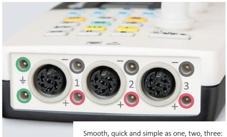
Smooth, quick and simple as one, two, three: record motor response using the first channel, sensory response using the second channel and needle EMG using the third channel.
